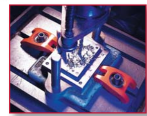
Working Height (H) Note that the bolt is always straight because of the swivelling pivot. Ranges from 0-75mm depending on model.
