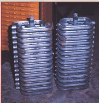
Stack Moulding of G-Clamp castings using chemically bonded sand to achieve good surface finish
